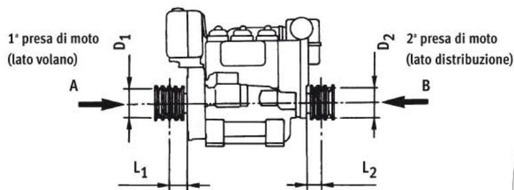
$$D_1 \text{ (mm)} \geq 100 [185 + L_1 \text{ (mm)}] \frac{N \text{ (kW)}}{n \text{ (RPM)}}$$
