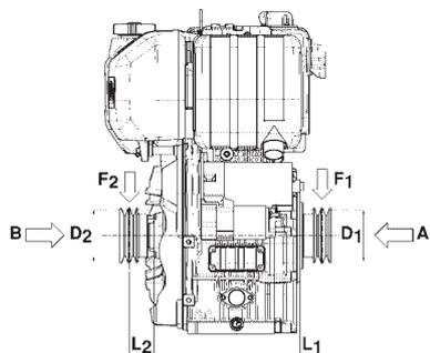
$$D_2 \text{ (mm)} \geq 860 [60+L_2 \text{ (mm)}] \frac{N \text{ (kW)}}{n \text{ (RPM)}}$$
